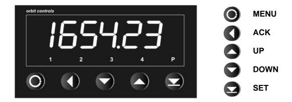
The key **MENU** opens the menu. The required parameter will be confirmed with **ACK** and set with **UP** or **DOWN**.
